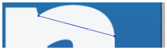
Here we have two spline points (in blue), and two tails (whose endpoints are in blue/white). By dragging the left tail end point upwards we see the spline take shape:
