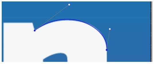
The end point of the tails can even by constrained. By adding a "vertical" constraint between the right spline point and the right tail end point, we can ensure that the spline is vertical there (constraint shown highlighted in orange):
